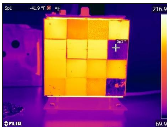
Figure 3.7. Thermal image captured using an LWIR camera, illustrating temperature variations across different materials [46]
