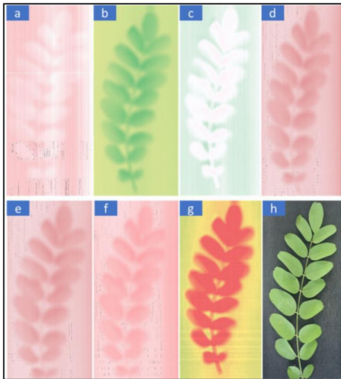
Figure 3.9. Comparison of the MS images. a) blue, b) green, c) red visible bands, d-f) infrared bands, g) full-spectrum reflectance, and h) the original image of a plant [48]
