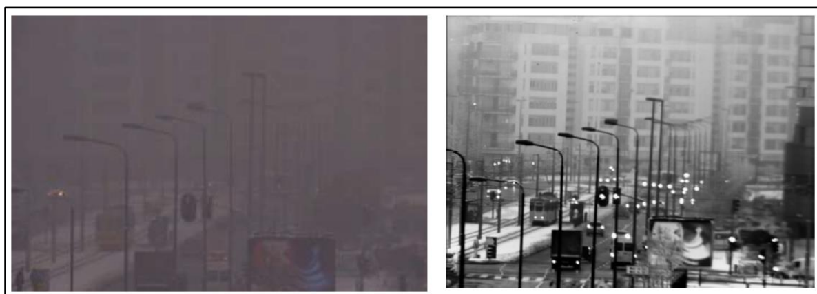
Figure 3.3. Comparison of visible light (left) and SWIR imaging (right) in low-visibility conditions. The SWIR image demonstrates to penetrate atmospheric interference [9]
